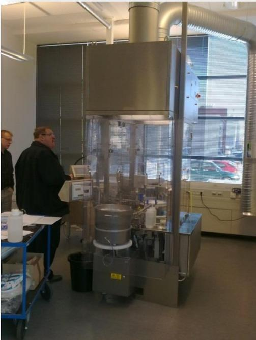
Picture 1. The air purifier is installed and connected to a dispensing machine
