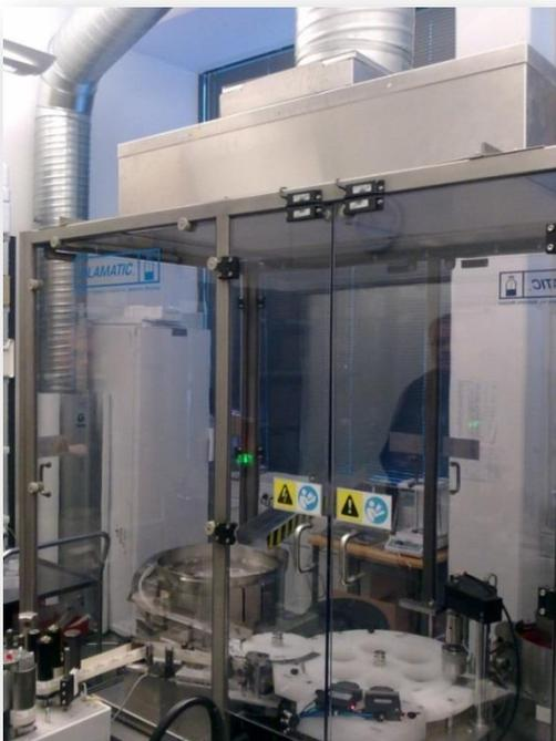
Picture 3. Cabinet of a dispensing machine with pure air connection (on top) from Genano® air purifier Source: Courtesy of Genano and Finnzymes, Finland.
