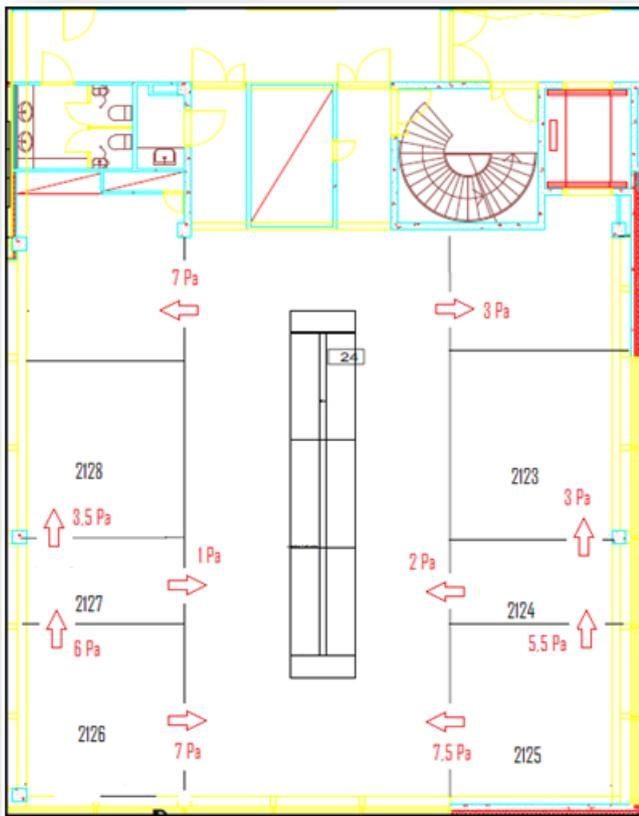
Three different air purification solutions were installed to laboratory premises depending what is the desired cleanliness level. In the picture is the layout of the laboratory. The laboratories equipped with Genano solution are in decreasing cleanliness level 2125, 2126 and 2123.
